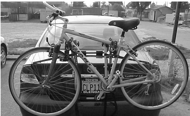
Fig. 7: On a bike with a slanted top tube, place top tube on rear cradle, and down tube on front cradle to keep bike as “level” as possible.
